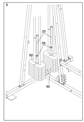
Lubricate the insides of the holes in the Top Weights (24) as shown. Slide a Top Weight onto each set of Weight Guides (23).
